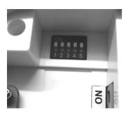
To adjust the RF address code of the Control Centre, remove one or more of the jumper caps located on the back of the unit (labelled 1,2,3,4 and 5, and shown in the picture below) so that the jumper settings match the settings made on the receiver:
